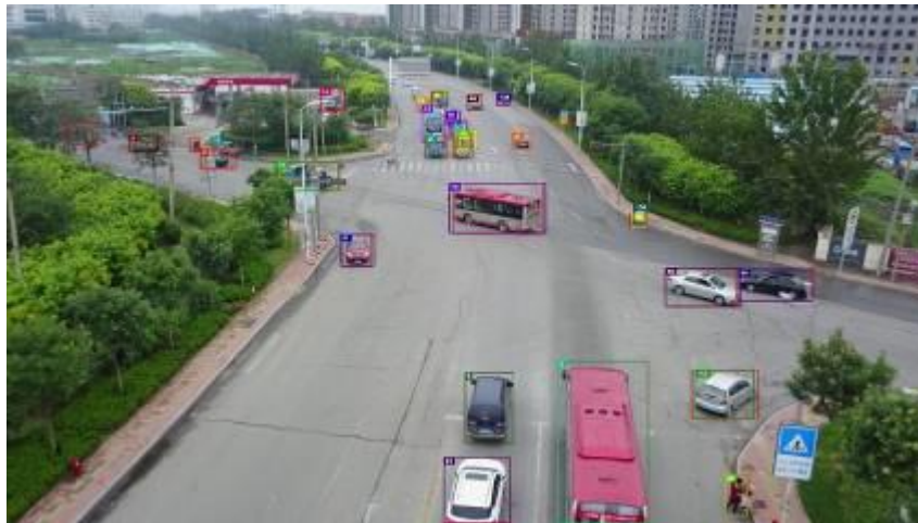
Figure 15. Sample frame with tracking results of one the sequences of the VisDrone 2018 dataset. Numbers stand for the identifiers of the tracked vehicles.
